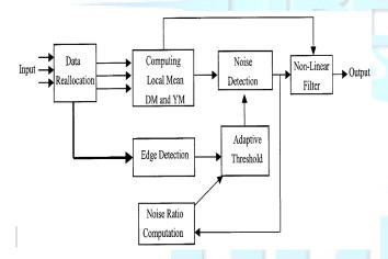
Fig. 2 Noise Reduction Architecture
